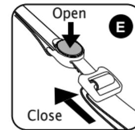
The helmet must sit firmly and level on your head. Lower the front of the helmet to cover your forehead by tightening the chin strap and loosening the rear strap. To uncover your forehead, loosen the chin strap and tighten the
