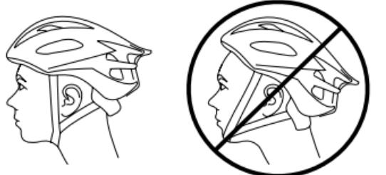
To check proper strap tension, put on the helmet and fasten the buckle. Open your mouth. You should feel the strap pulling against your chin. Then try taking off the helmet by pulling it forward and backward. If the helmet comes off, increase the strap tension. The helmet should not move excessively. It should not be possible to take off the helmet without unfastening the buckles.
